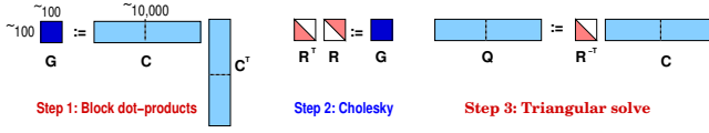
Figure 4: Illustration of CholQR on two GPUs, where the dashed lines show the matrix distribution.
