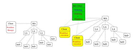
Figure 5: Software architecture of DIET workflow engine.
