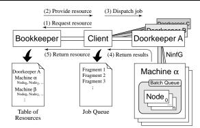
Figure 23: Structure of the middleware composed of Ninf-G.
