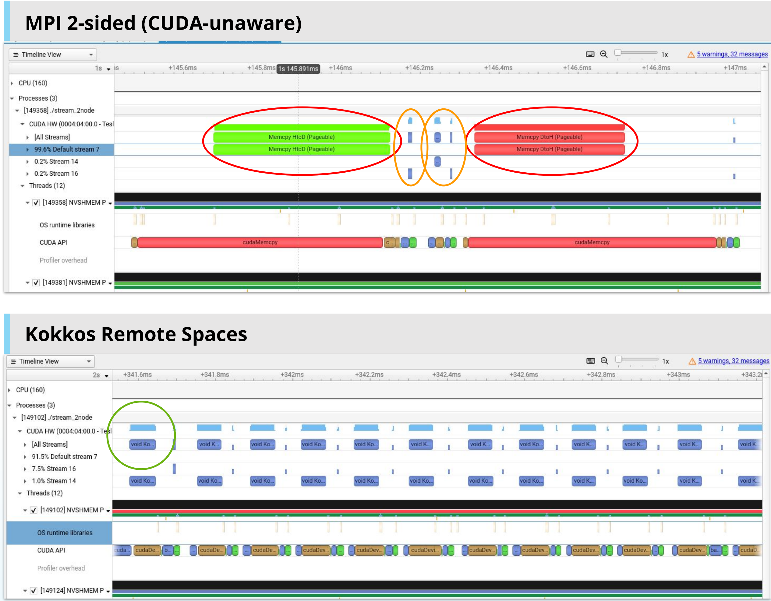
Above: traces visualized with NVIDIA Nsight that show time taken for host-device transfers that can be skipped with device-device communication exposed through Kokkos Remote Spaces.
