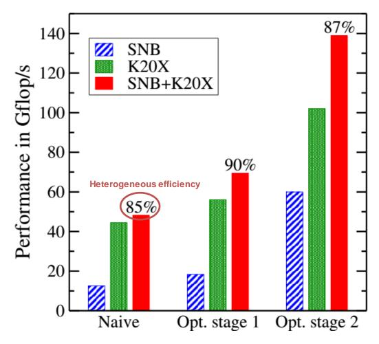
SNB: Intel Xeon E5-2670 "Sandy Bridge", K20X: Nvidia Tesla K20X, Complex double precision data (topological insulator)
