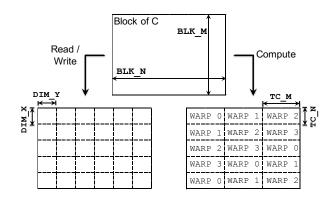
Fig. 3. An example for the double-sided recursive blocking applied to a block of C. The blocking dimensions for reads and writes are decoupled from those used for computations. The right side also shows how four warps can collaboratively work on a block og C.
