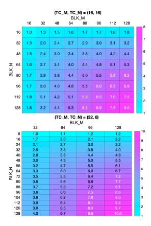
Fig. 5. The relative reduction in memory traffic for A and B using (BLK\_M, BLK\_N)  $\geq$  (TC\_M, TC\_N). Results are shown for (TC\_M, TC\_N) = (16, 16) "top," and (32, 8) "bottom.." Note that BLK\_x must always be multiple of TC\_x.
