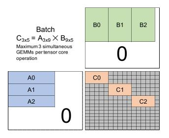
Fig. 10. Improving Tensor Core utilization by assigning multiple GEMMs at a time. Example for  $(M,\,N,\,K)$  =  $(3,\,5,\,9)$ , with all tensor core sizes set to 16.
