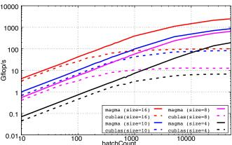
Fig. 17. Impact of batchCount on performance. Results are shown for very small selected sizes a Tesla  $V100\ GPU$
