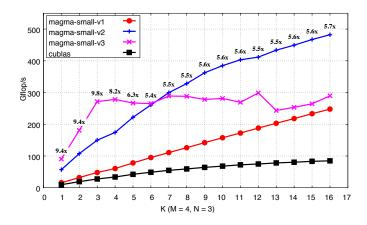
Fig. 15. Performance of all kernel versions against cuBLAS, with M=4 and N=3. Results are shown for <code>batchCount=1M</code>, on a Tesla V100 GPU
