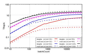
Fig. 16. Impact of batchCount on performance. Results are shown for selected square sizes on a Tesla  $V100\ GPU$
