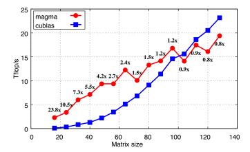
Fig. 7. Performance of the batched HGEMM kernel against cuBLAS. Results are for square sizes up to 128, with <code>batchCount = 50,000</code>, on a Tesla V100 GPU.
