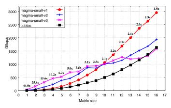
Fig. 13. Performance of all kernel versions against cuBLAS. Results are shown for square sizes up to 16, with batchCount = 1M, on a Tesla V100 GPU
