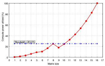
Fig. 14. The percentage of available Tensor Core compute power for square multiplications of small matrices.
