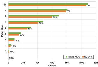
Fig. 8. Performance of the MAGMA kernel against against different values of NSG. Results are shown for square sizes up to 10, with batchCount = 1M, on a Tesla V100 GPU.
