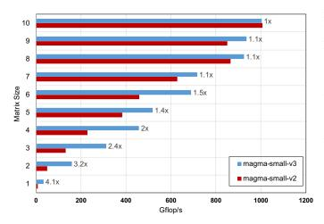
Fig. 12. Performance improvement of magma-small-v3 against magma-small-v2. Results are shown for square sizes up to 10, with batchCount = 1M, on a Tesla V100 GPU.
