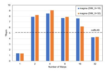
Fig. 4. The impact of the number of warps on performance for relatively large blocking sizes. Results are shown for square  $64 \times 64$  matrices using a Tesla V100 GPU, with batchCount = 50K. All blocking sizes are set to 64, with all Tensor Core sizes set to 16. DIM\_Y = (#warps $\times$ 32)/DIM\_X.
