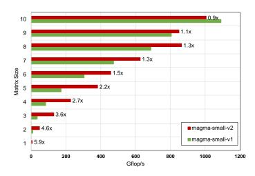
Fig. 11. Performance improvement due to increased Tensor Core utilization. Results are shown for square sizes up to 10, with batchCount = 1M, on a Tesla V100 GPU.
