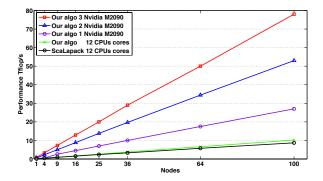
Figure 2. Weak scalability (horizontal reading) strong scalability (vertical reading) of the distributed multi-device Cholesky factorization on System A.
