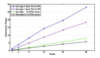
Figure 4. Weak scalability (horizontal reading) strong scalability (vertical reading) of the distributed multi-device Cholesky factorization on System B.
