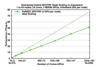
Figure 9: Performance of DPOTRF using distributed GPUs.
