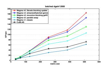
Fig. 9. Performance in Gflops/s of our different version of the batched LU factorization compared to the CUBLAS implementation.
