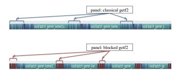
Fig. 5. Execution trace of the batched LU factorization using either classical getf2 (top) or our recursive getf2 (bottom).
