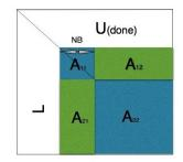
Fig. 1. Access patterns to matrix regions for the blocked right-looking LU factorization algorithm.
