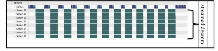
Fig. 7. Execution trace of the batched LU factorization using either batched dgemm (top) or streamed/batched dgemm (bottom).
