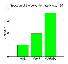
Fig. 10. XNET Solver speedups using either the sparse solver MA48 or our MAGMA batched LU factorization on a K20x GPU versus the MKL library.
