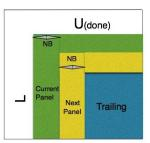
Fig. 2. Access patterns to matrix regions for the recursive blocked algorithm.
