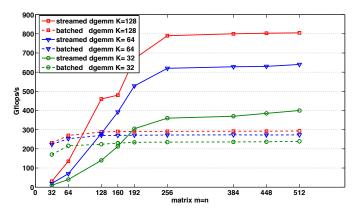
Fig. 6. Performance comparison between the streamed and the batched dgemm kernel for different value of K and different matrix sizes where m = n.
