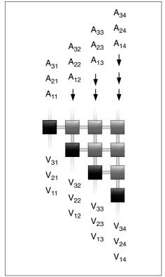
Figure 3. Systolic array for tile QR.
