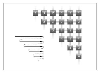
Figure 5. Mapping of systolic units to cores.
