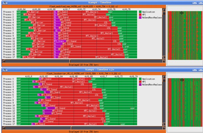
Figure 3: Typical communication pattern in the FLASH code. An MPI\_Barrier call before a communication phase ensures a synchronized start of the communication calls (top). When removing the barrier there is an un-synchronized start (bottom). Yet, this imposes no additional time on the following MPI operations, the runtime per communication phase is reduced by approximately  $1/3$ .
