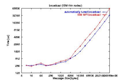
**Figure 3.** FT-MPI tuned collective broadcast versus IBM MPI broadcast on IBM SP2 thin node system.
