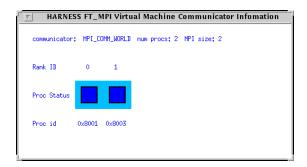
**Figure 9.** Cominfo display for the above application after a communicator rebuild using the SHRINK option. Note the communicator status box has changed back to a blue (dark) colour.
