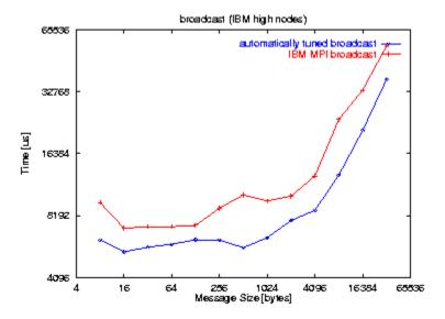
Figure 4. FT-MPI tuned broadcast versus the IBM MPI broadcast on an SP2 high node system
