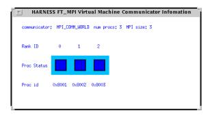
**Figure 7.** Cominfo display for a healthy three process MPI application. The colours of the inner boxes indicate the state of the processes and the outer box indicates the communicator state.
