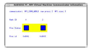
**Figure 8.** COMINFO display for an application with an exited process. Note that the number of nodes and size of communicator do not match.
