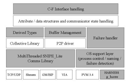
Figure 1. Overall structure of the FT-MPI implementation.
